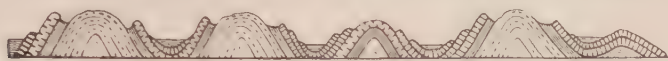
FIG. 344. — Section through the Juras, showing mountain ridges produced by several open folds, like great earth waves.
